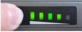
The state of charge of the battery you can control on the integrated display on the battery, when you push the red button. The battery is empty if only the red lamp is light.
