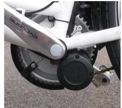
The motor is mounted in the bottom bracket instead of the bottom bracket.
