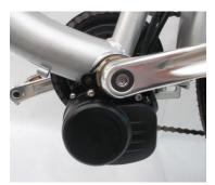
The nominal speed is 90 revolutions per minute, the nominal performance is 250 Watt and the maximal performance is app. 400 Watt.
