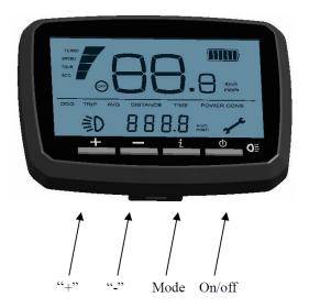
① Press this button to power on the LCD display, Long pressing the button for 2 seconds to power off. Automatically shut off without any operation in 5 minutes.
