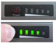
The state of charge of the battery you can control on the integrated display on the bat-
