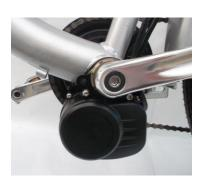
The nominal speed is 90 revolutions per minute, the nominal performance is 250 Watt and the maximal performance is app. 400 Watt.
