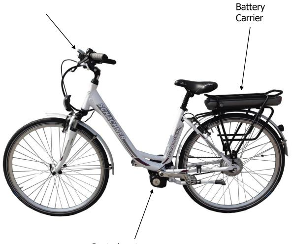
Central motor integrated controller Torque sensor
