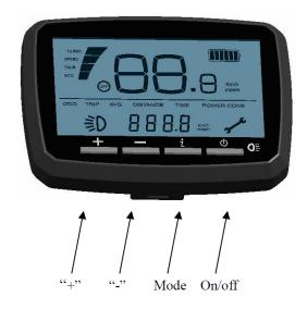
(h) Press this button to power on the LCD display, Long pressing the button for 2 seconds to power off. Automatically shut off without any operation in 5 minutes.
