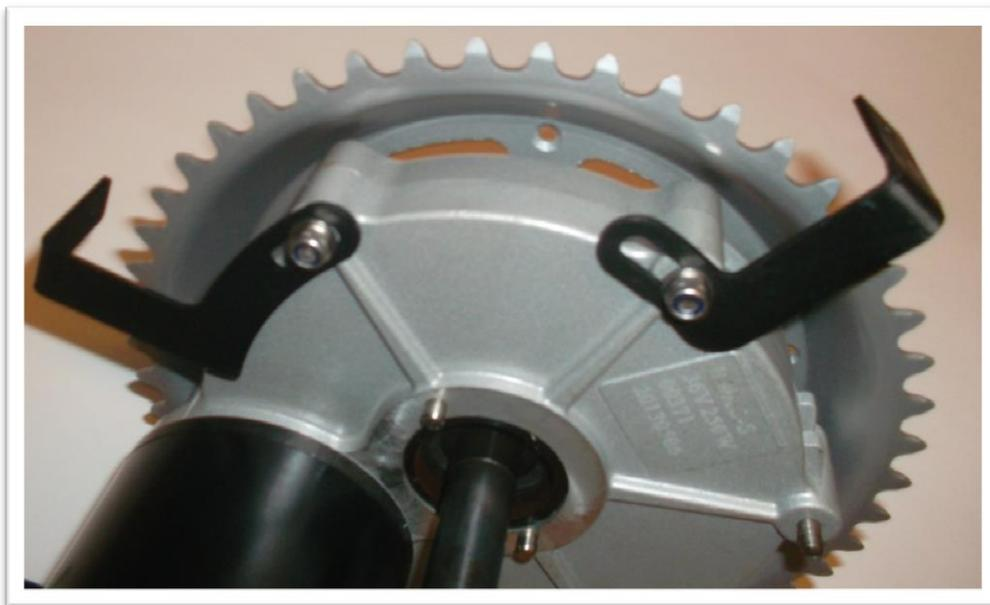
Lubricate the mounting tube and the axis of the engine with a heat-resistant, tough multi-purpose grease!
