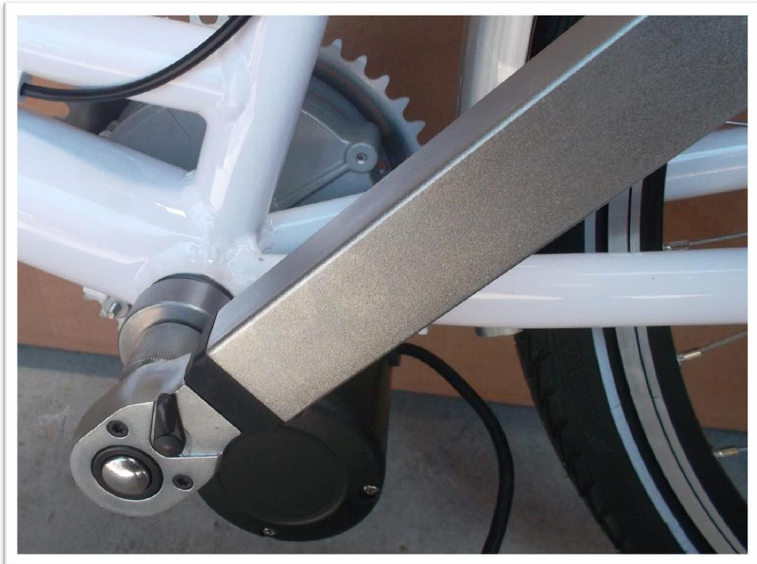
Pull the mounting tube with a torque of 85Nm fixed!
