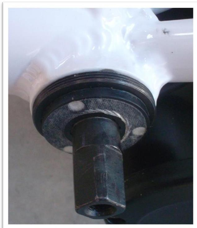
Now you can attach the magnetic disc cover. Look again on the free movement of the magnetic disk! Screw not too tight, as this is the only cover around an optical cover and is not intended to fix the engine!
